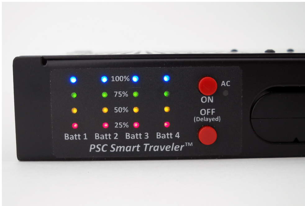
Close up of main unit battery monitoring and power buttons.
