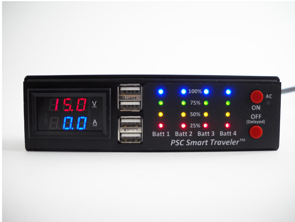
Remote Control showing output Voltage and Current Metering, USB Power Outputs, Battery Monitoring, Power Buttons.
